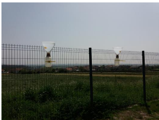
Fig. 1 – Sampling system composed of a funnel connected to a bottle (systems a and b), used to collect total atmospheric wet and dry deposition.
