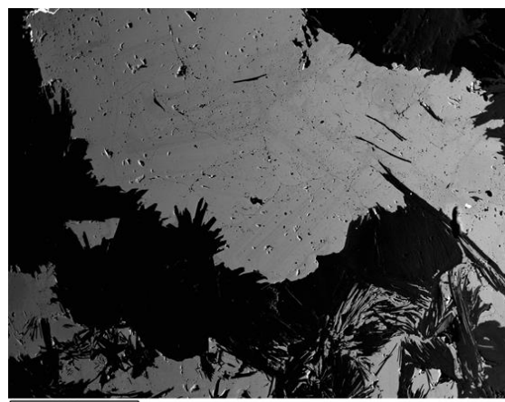
Fig. 4 - Backscattering image of selvage apatite crystals showing oscillatory zoning.
