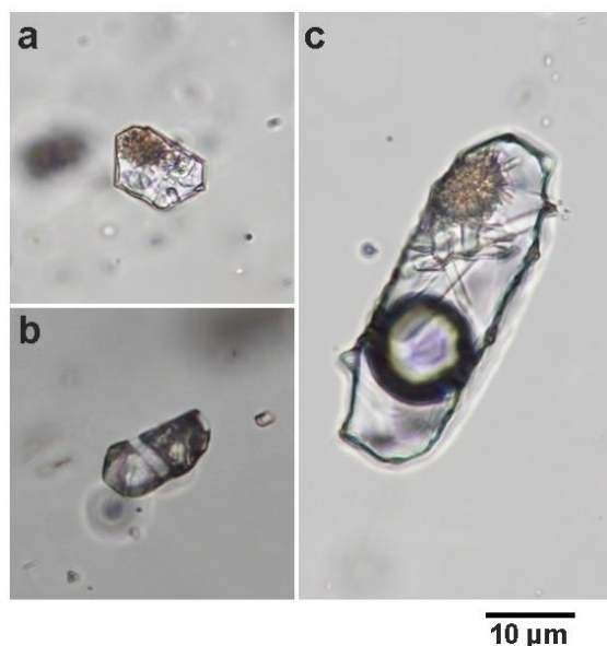
Fig. 5 – Examples of studied melt inclusions. Inclusions with no visible fluid phase (a, b) and fluid-rich melt inclusions (c).
